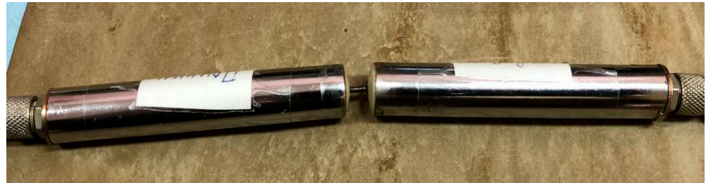
Figure 13. Photo of interconnected transducers.
