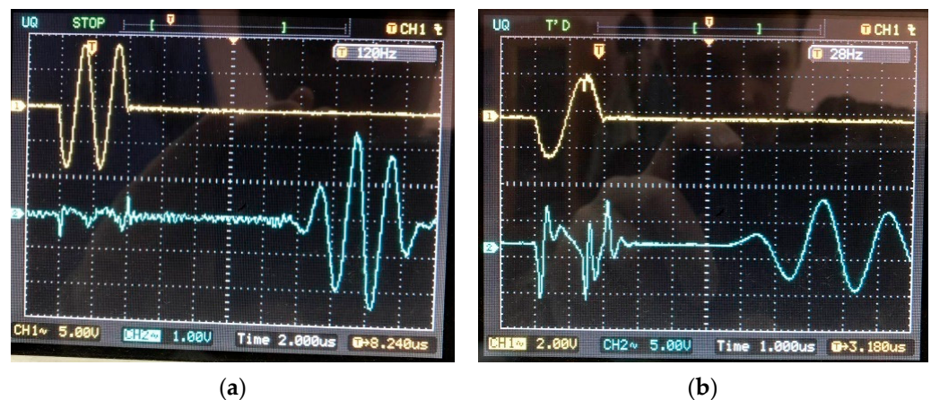
Figure 12. Oscillograms of signals: (a) during the study of the wave velocity; (b) with connected converters.
