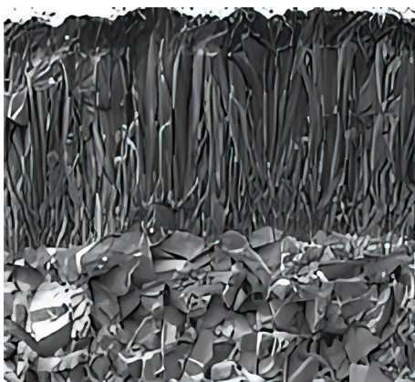
Figure 2. Microstructure of the surface of carbide cutting plates with TiN coating ( \times 1800 )
