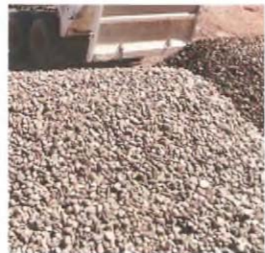
Gravel – coarse aggregate
