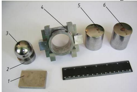
Fig. 3. Appearance of a device for measuring impact force by the elastic contact method: 1 - plate; 2, 5, 6 - punches; 3 - ball; 4 - case
