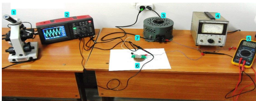
Fig. 1 – Appearance of the experimental setup for electroplasmolysis research: 1 – MICROMED biological microscope; 2 – digital oscilloscope; 3 – laboratory autotransformer; 4 – millivoltmeter; 5 – digital multimeter MY-64; 6 – experimental sample of vegetable raw materials; 7 – shunt for current measurement
