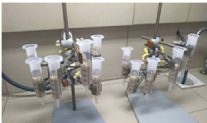
Figure 2. Sand columns for biocementation.
