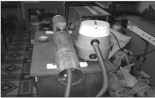
Laboratory aerodynamic unit for the study of wind erosion resistance of soil
